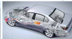
Waste Heat Recovery
